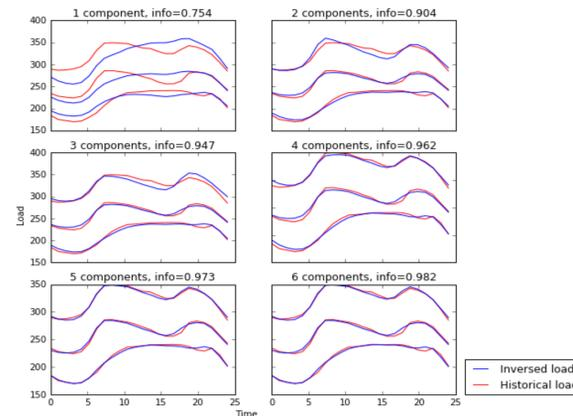
Fig. 3 Reconstructed hourly load profiles based on PCA
