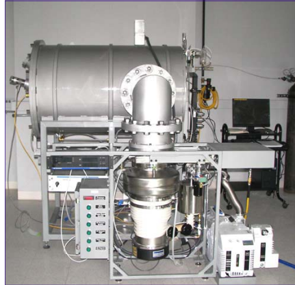
The new 3KW 30-inch diameter microwave firing chamber offers controlled atmosphere or vacuum with temperature monitoring using both optical pyrometry and thermocouple sensors.
