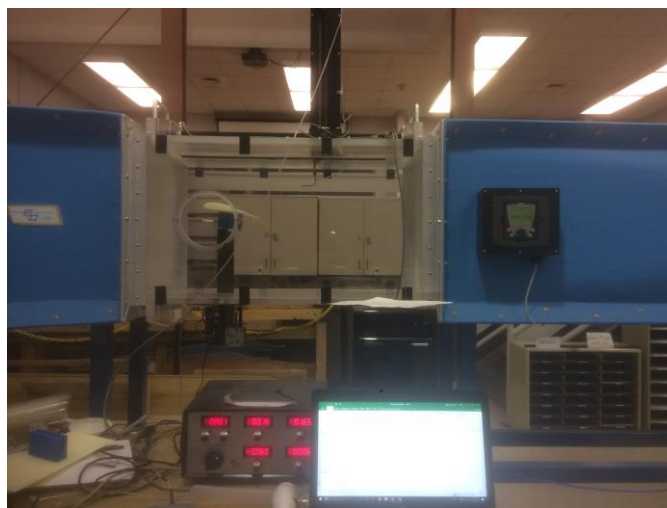
Figure 4: Wind tunnel testing equipment, with the control profile loaded at a 10° angle.
