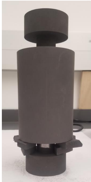
Figure 14. 1-inch inner diameter graphite die used for uniaxial hot pressing. Dies were lined with graphite foil of 0.005 inch thickness which was spray coated with aerosolized hexagonal boron nitride.
