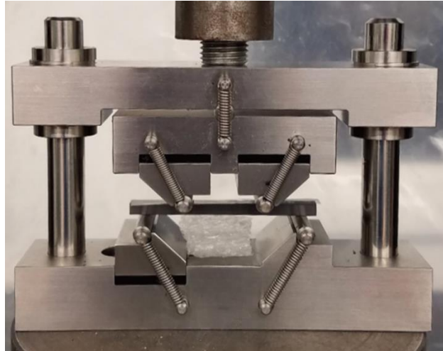
Figure 47. Experimental setup for four point \frac{1}{4} -pt flexure experiments.
