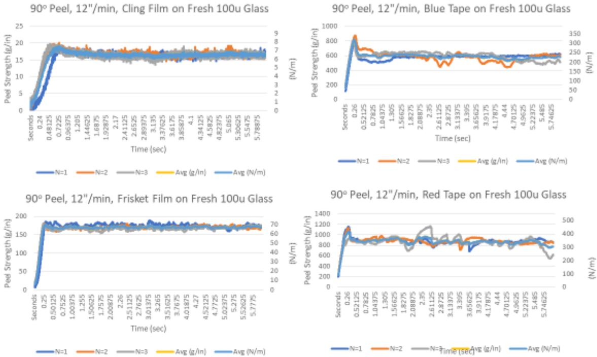
Figure 13 - Peel Strengths of Various Tapes / Films on Fresh Samples
