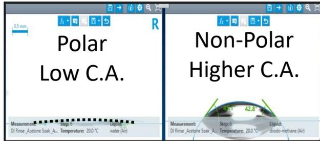
Figure 5 - Example of High vs. Low Contact Angle
