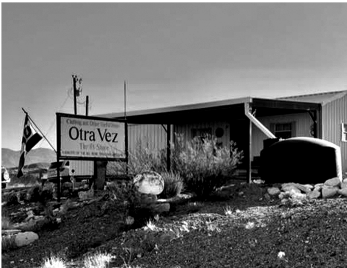
Otra Vez Thrift Store. Note the large tank on the right, which is a common sight in the desert. Most residents obtain their water supply by catchment, having designed their roofs to channel each precious drop that falls into such storage.
