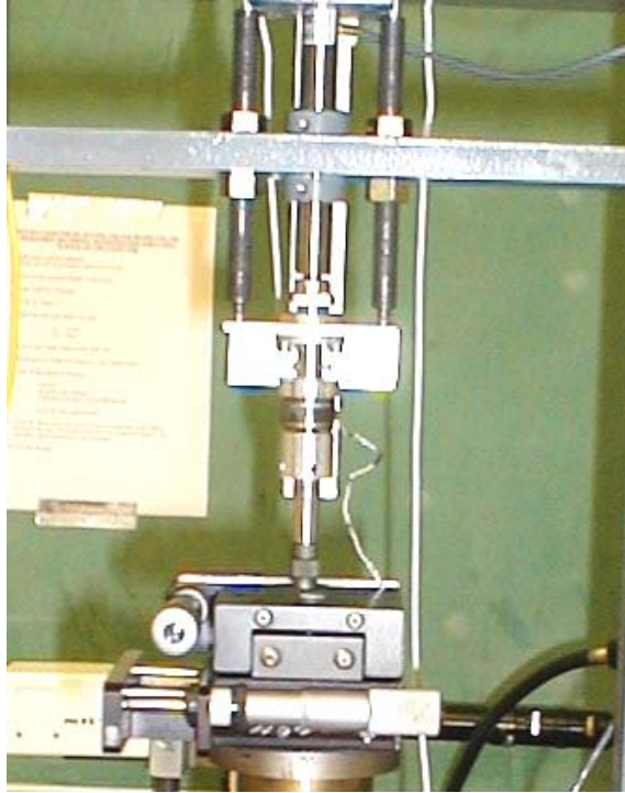
Figure 2.1. The dynamic recording microindenter used for this study. Shown in the top of the picture is the PZT column with dual capacitance gauges. The spherical indenter, sample and the translatable stage are also shown.
