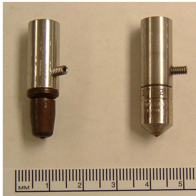
Figure 2.2. Indenters used for dynamic micro hardness measurements. Shown in the left is the 2mm ball indenter with hardened steel tip. Shown in the right is the 400 \mu m indenter with the diamond tip.
