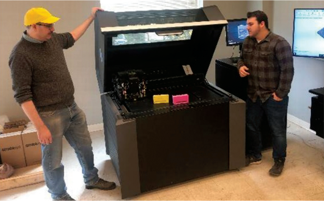
In the photo above, Steven Hyde, left, and Mark Ciccarella, senior ceramic engineering majors at Alfred University, observe two sample molds created in a 3-D printer at Replacement Tiles Solutions, where they work as research assistants. Replacement Tiles Solutions, located in the IncubatorWorks facility in Alfred, is commercializing a new additive manufacturing-based system for the terra cotta industry.
