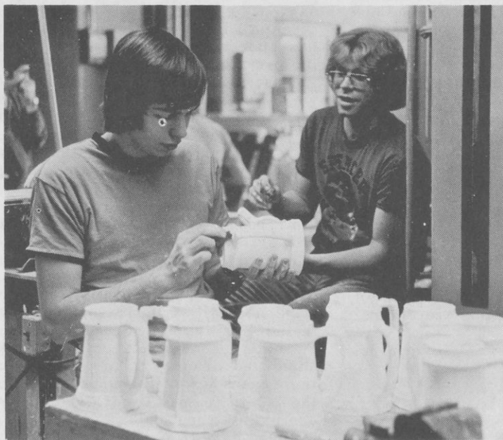
Mug makers smooth out rough spots before glazing and firing
