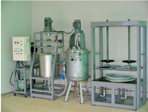
Pressure casting machines for pottery industries made by this company.
