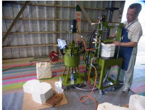
Pressure casting machines for pottery industries made by this company.
