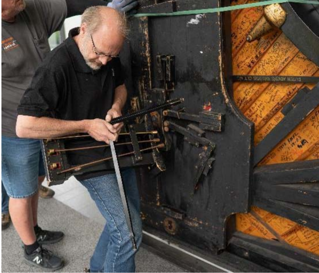
Nathan Baldwin, piano technician, installs the foot pedals on the Horowitz Steinway Piano.
