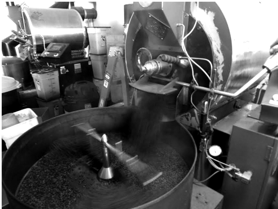
Twenty-three kilograms of hot roasted beans, accompanied by a puff of smoke, rush into the cooling sieve, instantly making a popping or "cracking" sound as they cool. (Photos by Sherry Volk)
