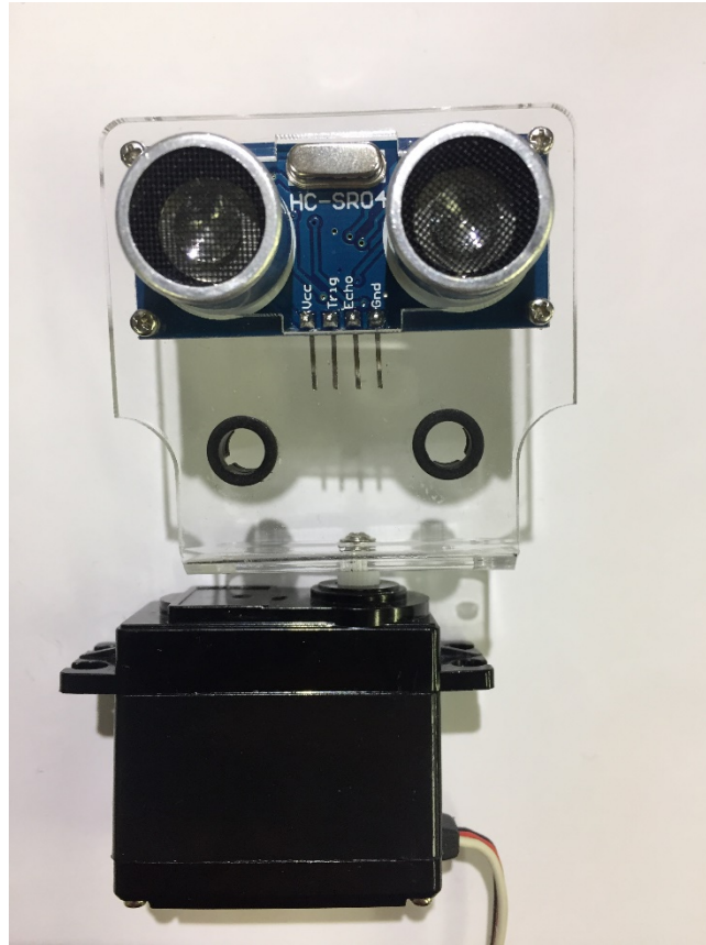
Figure 24. Ultrasonic sensor mounted on a servo.
