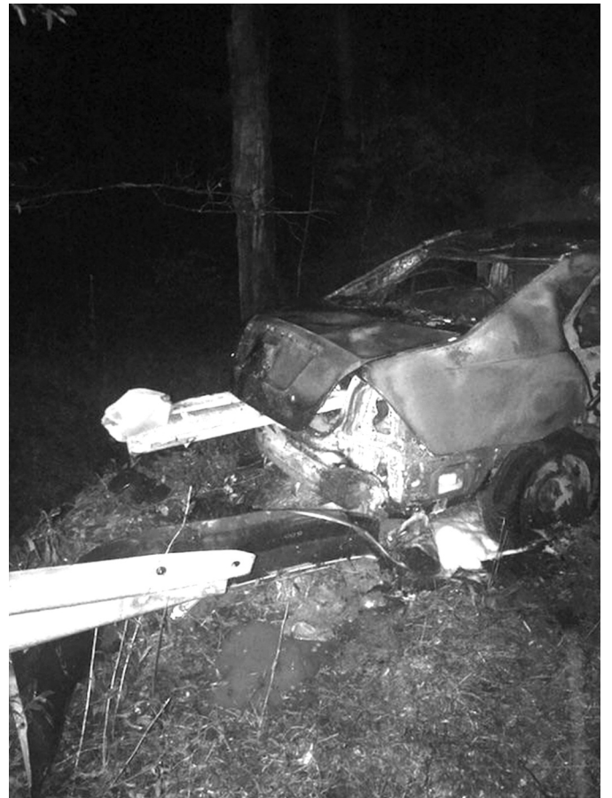
At left, front of vehicle was penetrated by guard rail, completely piercing the vehicle, coming out the trunk (right).
