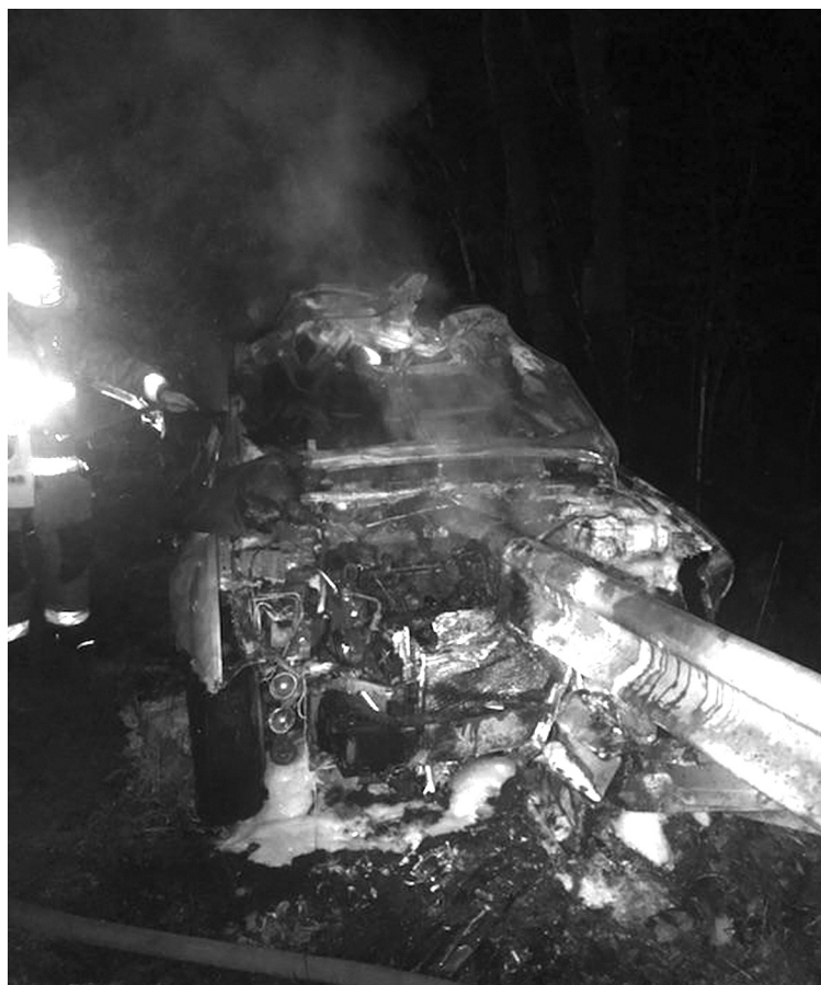
At left, front of vehicle was penetrated by guard rail, completely piercing the vehicle, coming out the trunk (right).
