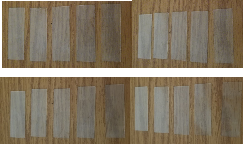
Figure 4. Set 1 (upper left), Set 2 (upper right), Set 3 (lower left), and Set 4 (lower right) with increasing grit going from left to right.
