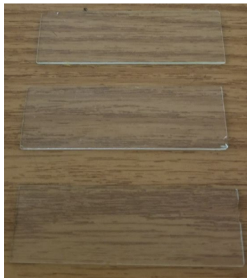
Figure 5. 3 glass slides, scratched with a dull knife (top), a sharp knife (middle), and cement (bottom).
