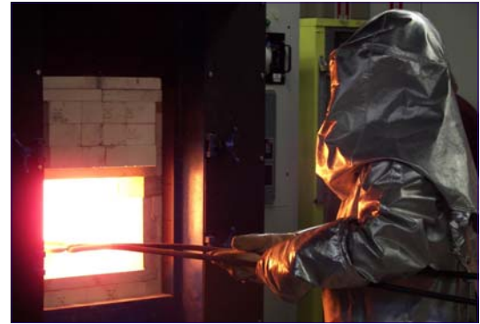
Above, each student manipulated the 4-foot-long tongs to extract the crucible of hot glass from within the over-1500°C furnace, transporting it to the pouring plate, below.
